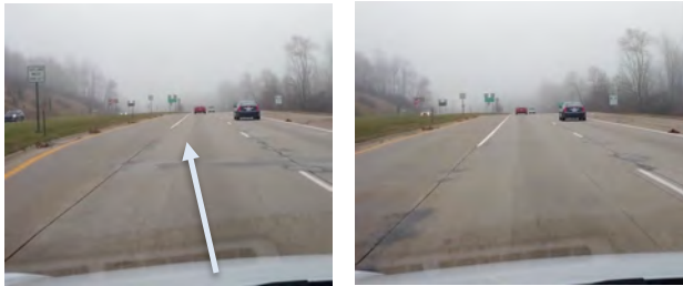
Figure 2: Disappearing lane markings & exiting (source tuan)
